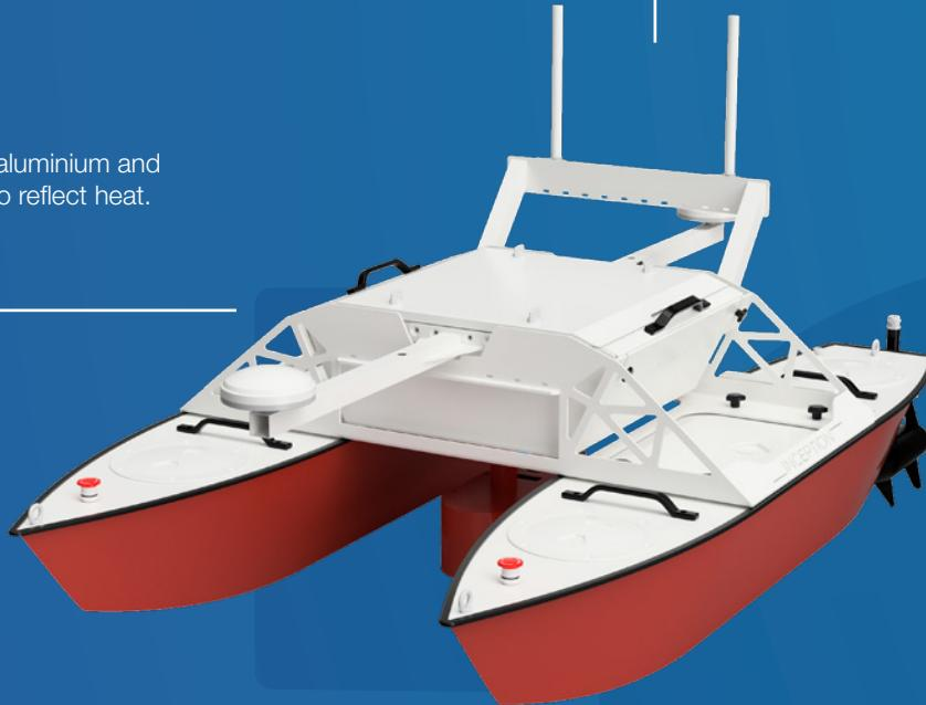
Twin aluminium hulls are robust, buoyant & stable.
